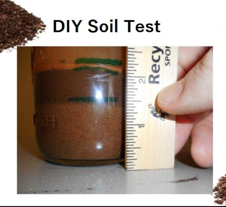
Silt Layer Height: 0.5" ÷ Total Height: 2.125" X by 100 to get % = 24% Silt
