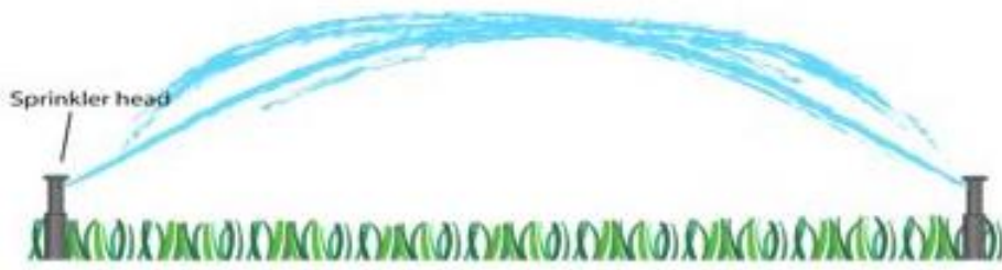
Area between heads is receiving the same amount of water.
