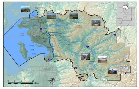
dam, then flows through the canal until it enters two large aqueducts along the Wasatch bench. Several creeks along the Wasatch Front can feed into this aqueduct system. From there, water is transported to each of the District's water treatment plants (WTPs). After complete treatment, water is delivered to cities or water improvement districts for final distribution to individual users.
